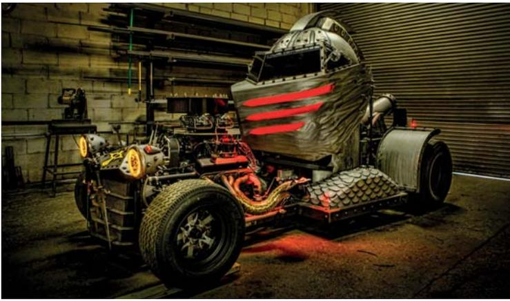
Starting as a re-skinned propane tank, Bohata designed the face shield and exterior himself. Hydraulic rams lift the mask, while the helicopter-like steering column swings out of the way for easy access to the seats.
