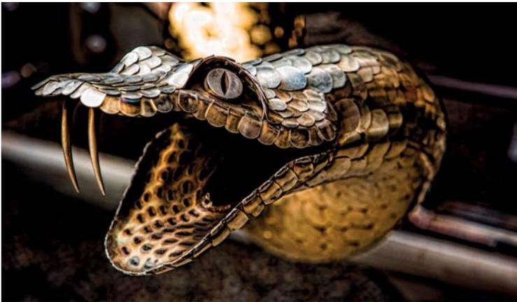
Each header is comprised of nearly 900 TIG-welded scales and also features CO2 blasters for local shows.
