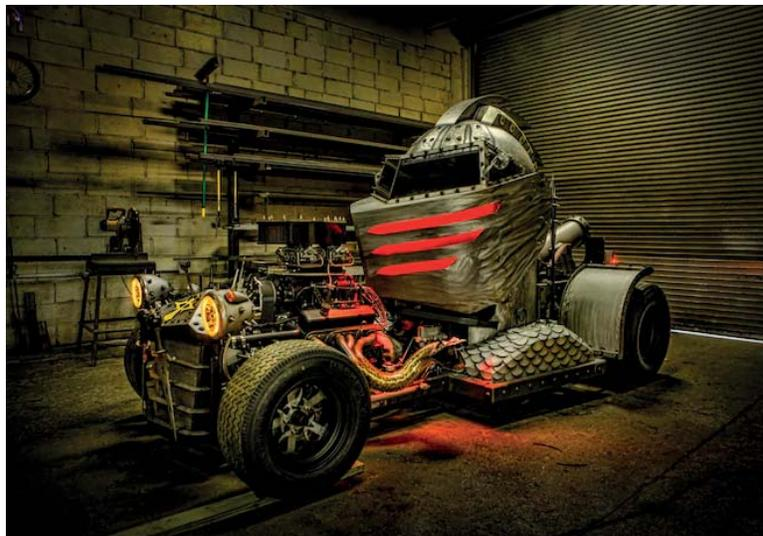
The chassis is laser cut from 2x4x3/16-wall rectangular tubing, jugged up and TIG-welded in-house. Up front, Medieval One uses a traditional drop axle with radius rods and a transverse monoleaf, while the rear axle uses air-ride suspension with stainless-steel axes flanking the wishbones.
